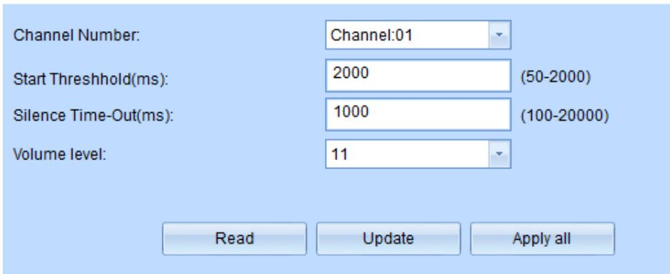
The user needs to configure sound level trigger level and sensitivity when the channel is set voice trigger recording.
